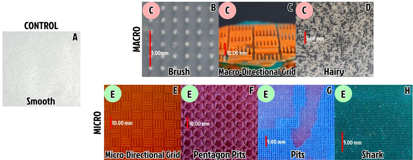
Figure 2: Castura Fabricated User Study Textures. A selection of textures that were fabricated via the *Castura* method. Textures marked with a "C" were fabricated with cut plates, while textures marked with an "E" were fabricated with an etched plate.
