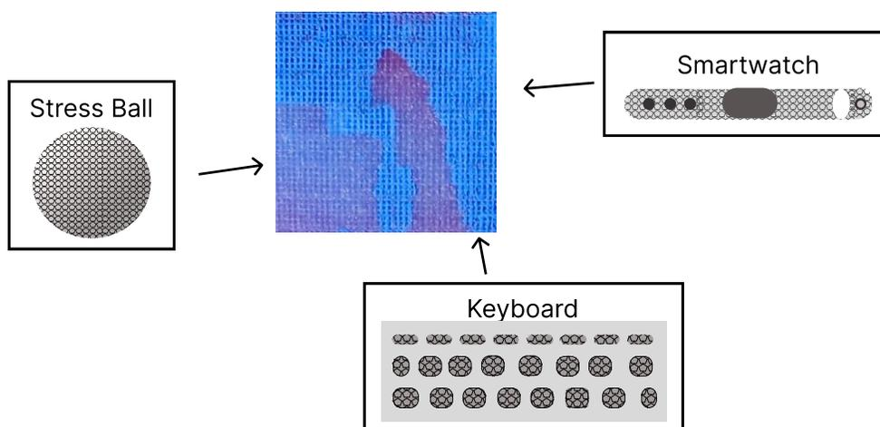
**Figure 1: The Pits Texture.** The Pits texture, made from cast silicone, features depression geometries of 0.53 mm by 0.5 mm and a spacing of 1.06 mm apart. A tap gesture was one of the preferred methods of stimulation, for which it was perceived as smooth, soft, silky, and fuzzy. Value could be found in applications such as wearable devices, haptic devices, and sensory devices.
