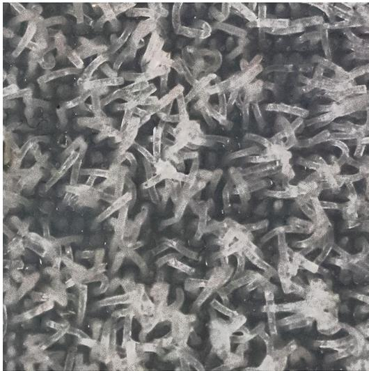
*Figure 1: A close-up image of one of the more intricate and detailed microtextures produced via the casting technique; users perceived this texture as 3.25 soft/hard, and 3.00 smooth/rough (5 pt Likert scale).*
