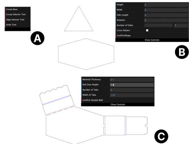
**Figure 3: Proto-Packs UI, polygon base, and double roll over functions (A) Blank canvas (B) Polygon base editing (C) Double roll over editing**
