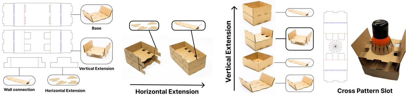
**Figure 4: (left to right) Dielines created in Proto-Pack with the corresponding folded component labeled. Example of *horizontal extensions* and *wall connections* being used to expand a package horizontally. Example of *vertical extensions* being used to expand a package vertically. Example of a *cross pattern slot* holding a non-planar shape within a package**
