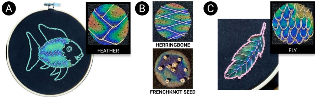
**Figure 10: Thermal Textures.** A) A rainbow fish design is illuminated with a visual and haptic fish scale texture using a feather stitch; B) the herringbone and frenchknot provide unique heat fence effects and haptic features; C) A feather is embellished with a fly stitch which provides a directional haptic feature useful for denoting sliding touch interactions.
