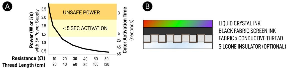
**Figure 2: LCTD Parameters. (A) Embroidered resistive heaters match well with the power and heat requirements needed to activate liquid crystal; (B) liquid crystal requires a black substrate to maximize the visual effect.**
