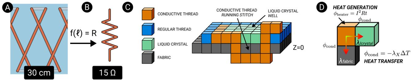
**Figure 3: LCTD Model.** A lumped model is constructed by (A) creating a physical model of stitches; (B) stitch length is converted to electrical resistance using a linear model; (C) a voxel grid is constructed from the physical model and used to (D) simulate heat transfer; conductive thread voxels generate heat according to Ohms' Law.
