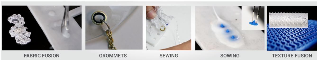
Figure 6: Five different fixturing techniques provided by Compressables Prototyping Toolkit to improve wearability.
