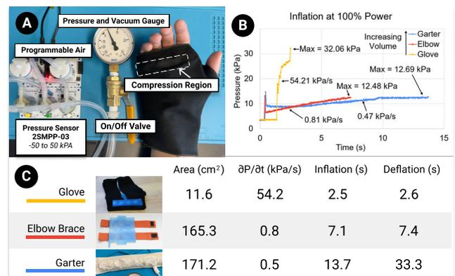
**Figure 10: Compressibles Pressure Characterization. A: Characterization Setup; B: Inflation Times at 100% pressure; C: Bladder Properties and Pneumatic Characteristics.**
