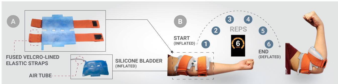
**Figure 7: Elbow brace.** A: An air bladder is fused with velcro-lined elastic straps and worn on the inside of the elbow joint; B: The inflated bladder tracks bicep curls and deflates upon completion of a set.
