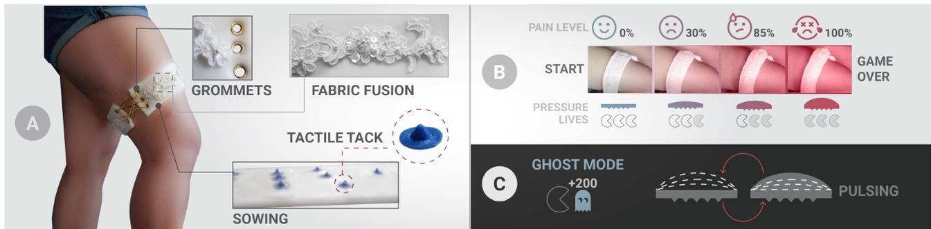
**Figure 9: Garter. A: An air bladder sowed with tactile tacks is held around the thigh using a gold chain; B: The bladder inflates on loss of life in a Pacman game and deflates on game over; C: The bladder pulses in ghost mode.**
