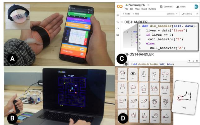
**Figure 11: User Study Setup. A: Users tested behaviors using the designer app and a tacked velcro-bound spherical compressable; B: Users integrated their behaviors to our API using Google Collaboratory; C: Users played Pacman to test their behaviors; D: Users brainstormed design potential and interaction ideas for different body parts**
