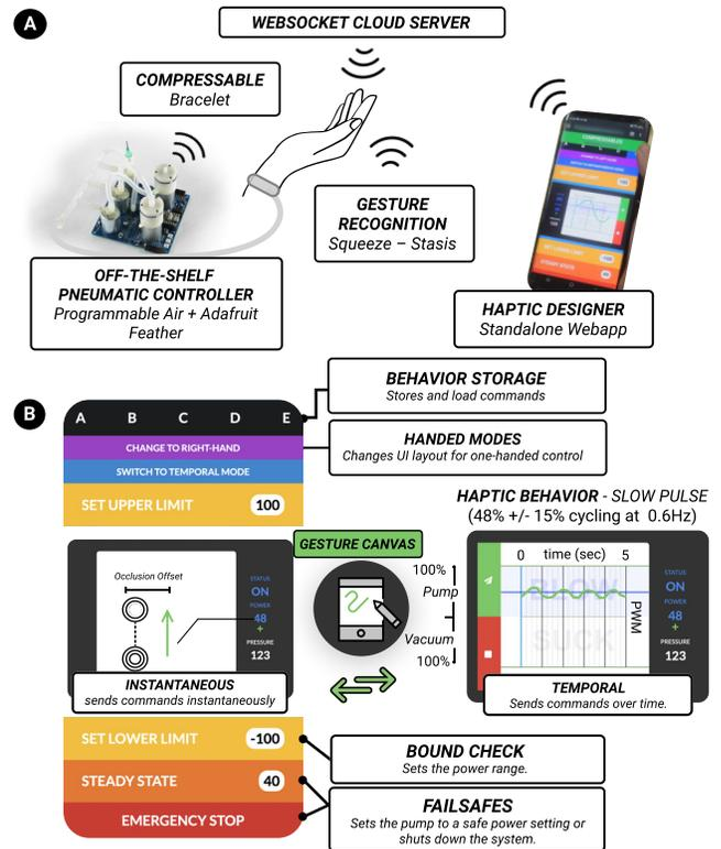
**Figure 3: Compressables Prototyping Toolkit. A: An off-the-shelf pneumatic controller is attached to a compressable bracelet using an air tube; all components intercommunicate using a websocket-based IoT server; B: A haptic design tool allows users to sketch compression-based behaviors and control the worn compressable.**
