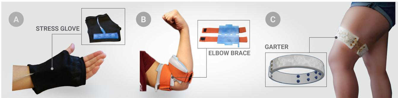
**Figure 1: Compressables.** A: An air bladder fused inside a fingerless glove inflates to provide stress-ball like interaction; B: An air bladder is fused with elastic straps to wrap around the elbow joint to track reps during exercise; C: An air bladder fused with lace and studded with tacks is wrapped around the thigh to provide an immersive gaming experience.
