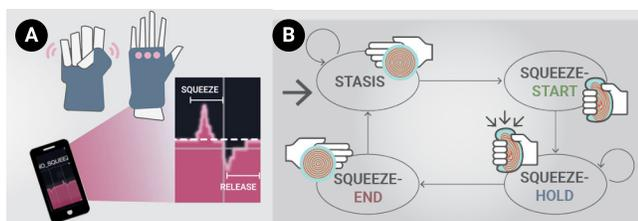
**Figure 8: Compressables State Machine for Squeeze Gesture.**
