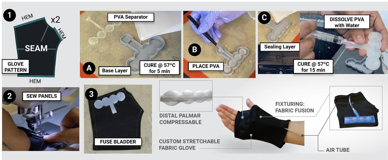
**Figure 5: The Making of a Stress Glove.** 1: A glove pattern is designed and laser-cut from fabric; 2: The laser-cut pieces are sewn together to form a fingerless glove; A, B and C: Silicone bladder fabrication (Section 5.1); 3: The bladder is fused to the glove using silicone as glue; Bottom right shows the final compressable.
