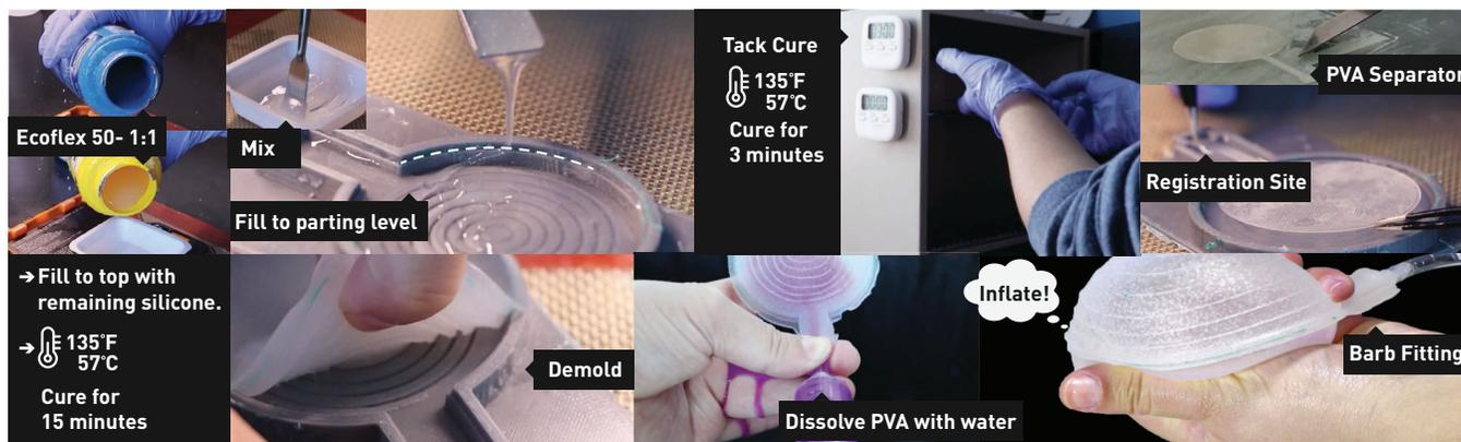
Figure 4. Bladder Fabrication Process. A single batch of silicone is prepared to fill a mold up to the parting level and speed cured to a tack state. A 3D-printed PVA separator is laid on the base layer, using a registration site to help anchor and align the element. The remaining silicone is poured and speed cured. Once demolded, the bladder is injected with warm water to dissolve the PVA and the resulting bladder is inflated.
