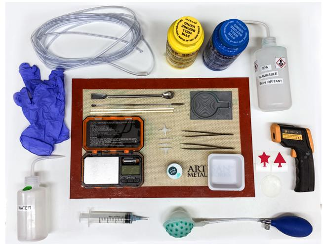
Figure 3. Materials, tools, and equipment used in bladder fabrication and testing. From bottom left, clockwise, moving inward: A water bottle, nitrile gloves, air tube, EcoFlex-50 silicone, isopropyl alcohol, an infrared heat gun, vinyl, polyvinyl acetate, an inflation bulb with valve, a syringe, a scale, glass rods, metal spatulas, molds, tweezers, antistatic weigh boats, silicone colorant, barbed airtube connectors. Not pictured: an FDM 3D printer, an incubator, and vinyl cutter.
