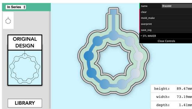
Figure 6. Design tool for silicone bladders. Given an SVG input, the separator and mold designs are procedurally generated.
