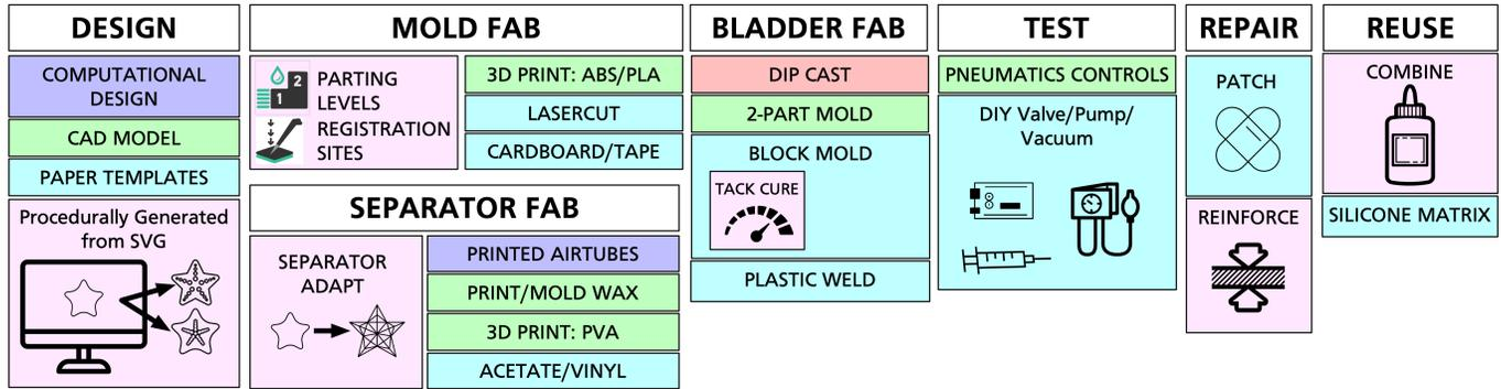
Figure 2. Diagram of how different Communities of Practices design and fabricate bladders. With Siloseam, we introduce both design and fabrication optimizations and methods of recombining, reusing, and repairing prototypes to support additional iteration cycles.
