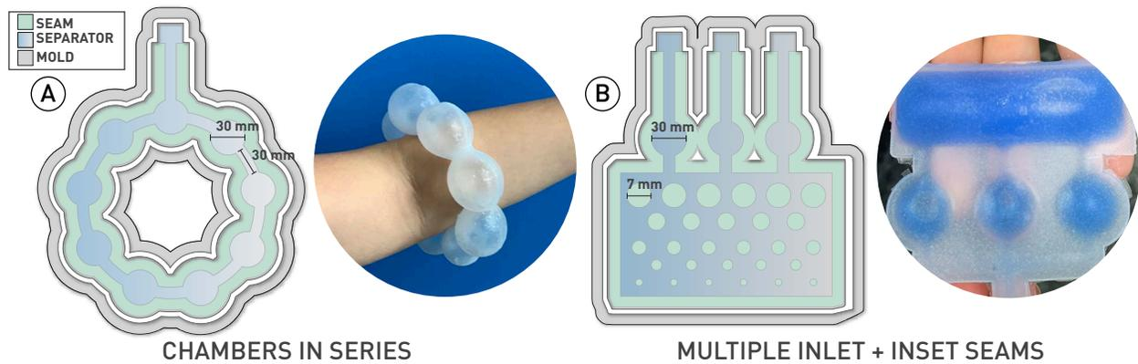
**Figure 8. Separator Design Patterns.** a) A nine-chamber bladder is connected with a single internal air channel; b) A three-chamber bladder is connected in parallel with a common sink chamber.
