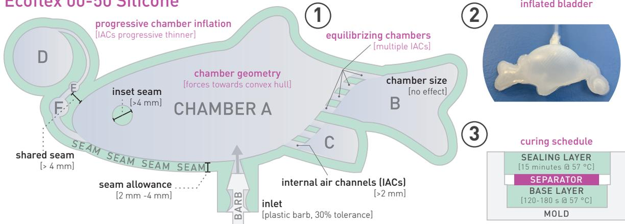
Figure 7. Bladder Design Guidelines for Ecoflex 00-50. 1) Anatomy of a bladder, 2) the bladder inflated, 3) the optimal curing schedule and layer and composition of the bladder.
