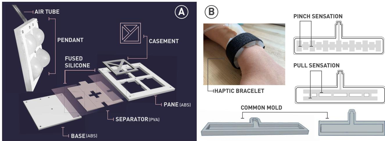
**Figure 9. Silicone Bladder Exemplars:** A) A mechanically-held seam necklace with interchangeable chamber designs, B) A bladder is fabricated from a common mold and used to prototype haptic sensations on the wrist.
